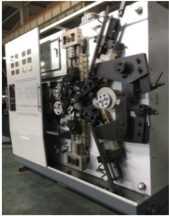
Automated cold coiling module TK-5200
