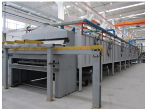
Through-type furnace for low-temperature tempering
