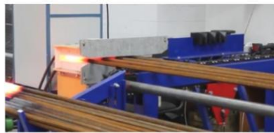
Through-type furnace for heating of rod ends
