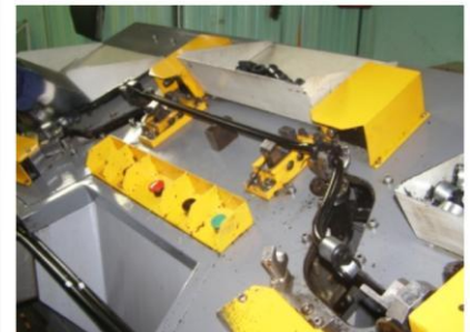
Stabilizer assembly with pads and links
