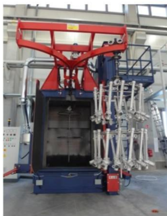
Shot- peening machine for stabilizer bars
