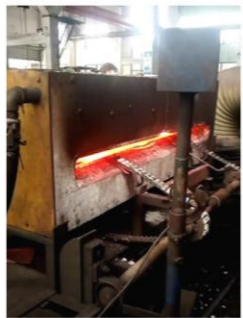
Slot furnace HFC for rod heating
