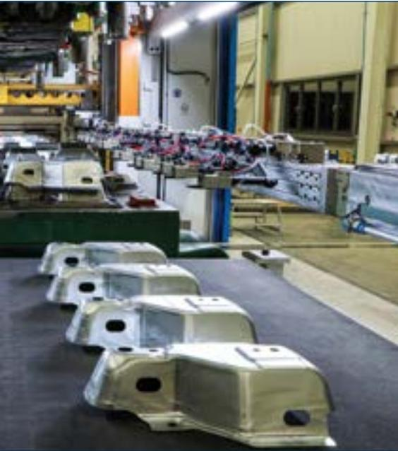
Production of pressed parts on modern stamping and forming technology. Photos: Vollmann Group
