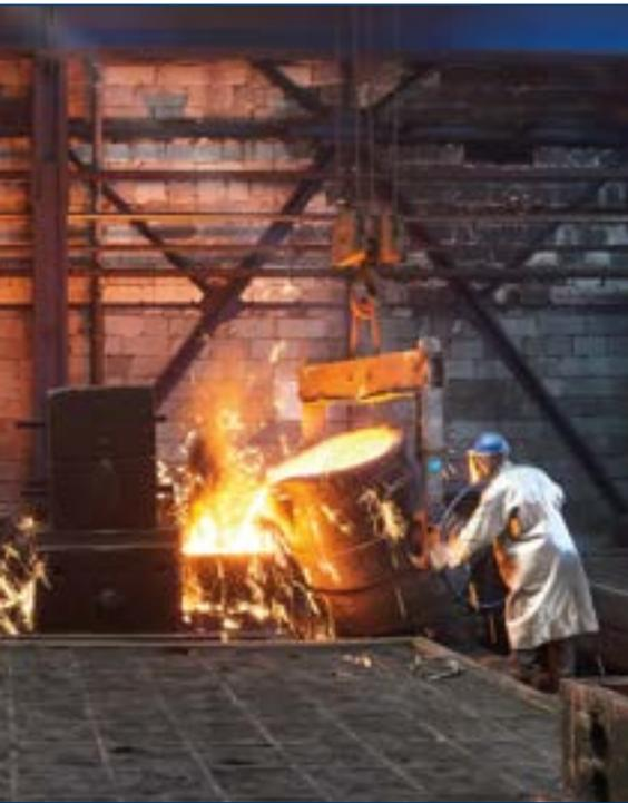
The production of vehicle bodies begins with the casting of press tool molds. The production of a state-of-the-art electric car, equipped with all of the latest software refinements, also begins with this physically tough and energy-intensive work. Gießerei Löbnitz is one of only a handful of foundries left in Germany that masters these processes.
